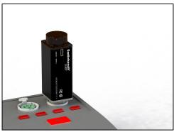
318BT can be connected directly to any XLR input (MIC Level), but before connecting; it is a good practice to ensure the Phantom Power is turned OFF on the input jack where 318BT is to be connected.
